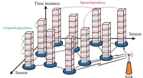
Fig. 1. A wireless sensor network with temporally and spatially correlated data samples with  $N = 10$  and  $T = 6$ .
