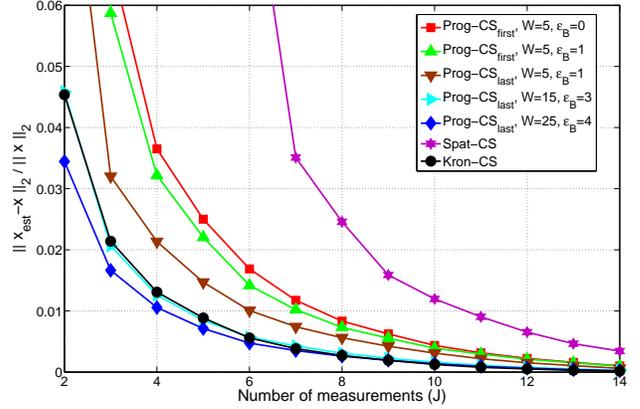
Fig. 2. CS recovery performance of Prog-CS, Kron-CS and Spat-CS.
