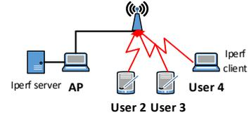
Fig. 1. Technology prototype topology
