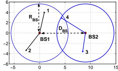
Fig. 1. MISO downlink wireless network with  $N = 2$  BSs and  $T = 4$  transmit antennas per BS.  $\mathcal{L} = \{1, 2, 3, 4\}$ .  $\mathcal{N} = \{1, 2\}$ ,  $\mathcal{L}(1) = \{1, 2\}$ ,  $\mathcal{L}(2) = \{3, 4\}$ .
