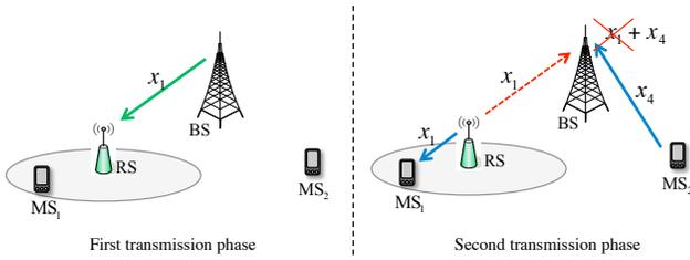
Fig. 1. CDR 1: relayed DL - direct UL. During the first transmission phase, BS transmits DL signal  $x_1$  to the RS. During the second transmission phase, two concurrent transmissions are scheduled: 1) RS transmits  $x_1$  to  $MS_1$  which causes interference at BS and 2)  $MS_2$  transmits  $x_4$  to BS. As BS knows  $x_1$ , the interference at BS can be cancelled.
