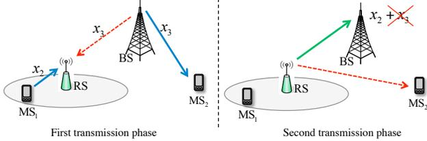
Fig. 2. CDR 2: relayed UL - direct DL. During the first transmission phase, two concurrent transmissions are scheduled: 1)  $MS_1$  transmits UL signal  $x_2$  to RS and 2) BS transmits  $x_3$  to BS which causes interference to RS. During the second transmission phase, RS transmits a signal containing  $x_2$  and  $x_3$  to BS (denoted generically as  $x_2 + x_3$ ). As BS knows  $x_3$ , the interference at BS can be cancelled.
