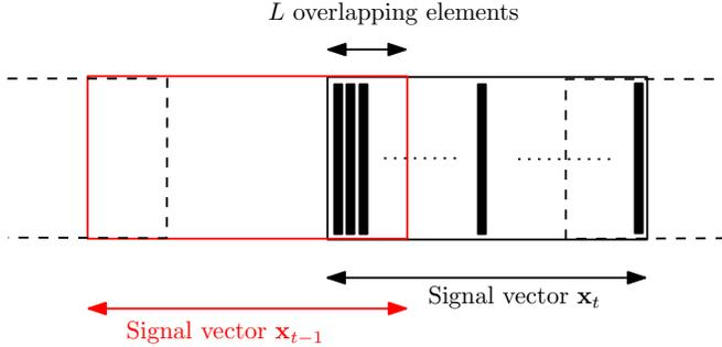
Fig. 1. Signal structure. Each signal vector  $x_t$  consists of  $N$  real valued elements. Each two consecutive signal vectors are overlapped each other.
