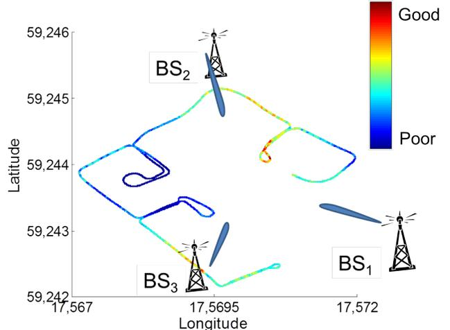
Fig. 1. Prediction errors were generated based the statistics of this drive route measurements from a suburb in Kista, Sweden.
